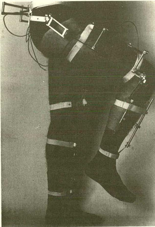
Figure 2. Side view of self-aligning goniometers for simultaneous flexion angle measurements of both hips and both knees, showing the method of attachment to thigh and shank, and the adjustable supports for potentiometers and linkage guides.
